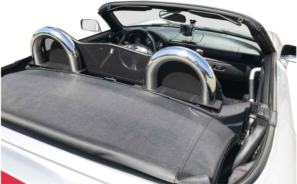
Attach the additional wind deflector using the supplied bolts. Install the plastic cap to cover the bolt.
